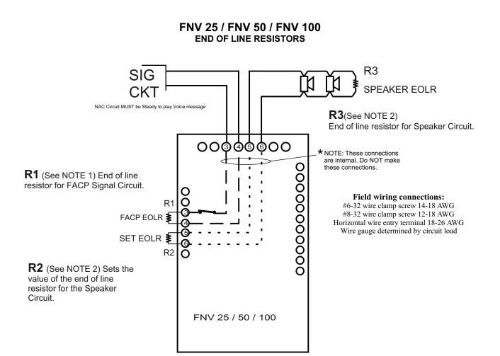
**NOTE 1**: If the Fire Alarm Signal Circuit requires a 4.7K end-of-line resistor, then R1 must be a 4.7K. Normally, this resistor is connected to the Signal Circuit through a closed Trouble contact. When the FNV 25/50/100 goes into Trouble, the contact opens, producing an "Open" on that Signal Circuit, notifying the FACP.
